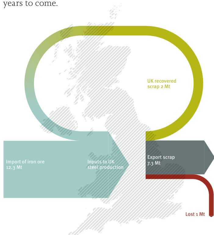
Current steel flows in the UK economy, from Completing the circle (June 2018)
